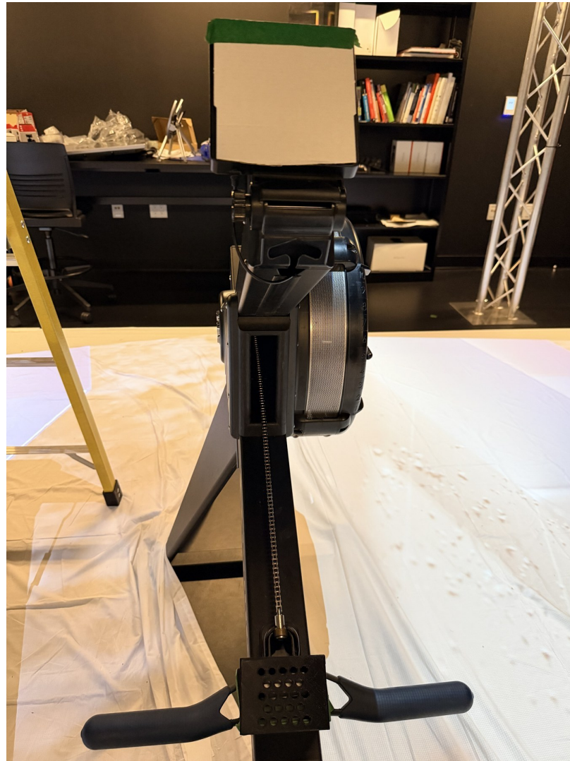
Figure 4.1: Instrumented ergometer, photographed with the room lights on for documentation; sessions ran with them off (Section 3.3). The white sheet serving as the projection surface is visible on the floor. The card cover withholds visible PM5 metrics during the recorded segment while Bluetooth telemetry continues; the dark handle-mounted housing contains the inertial unit (Figure 3.9).
