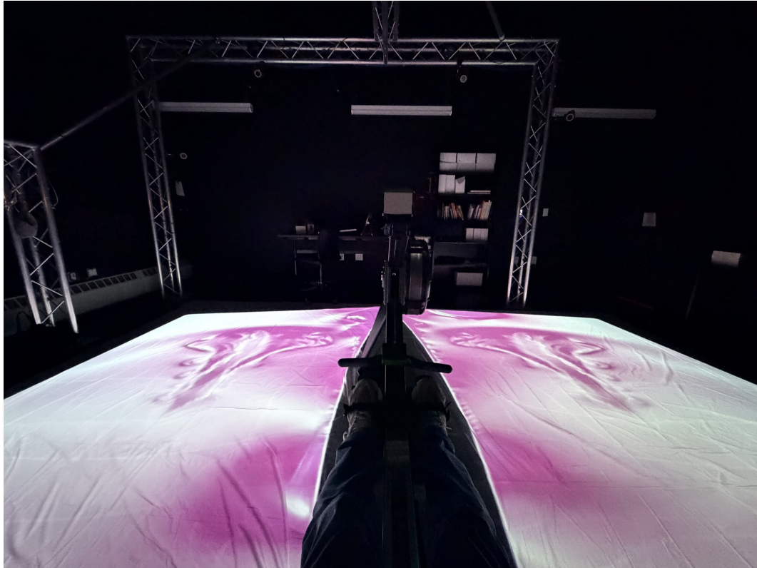
Figure 4.2: Participant-eye view from seated height. The ergometer and covered console occupy central vision, while the projection extends below and to both sides in the lower periphery. During recorded rowing it was the only visible feedback channel.
